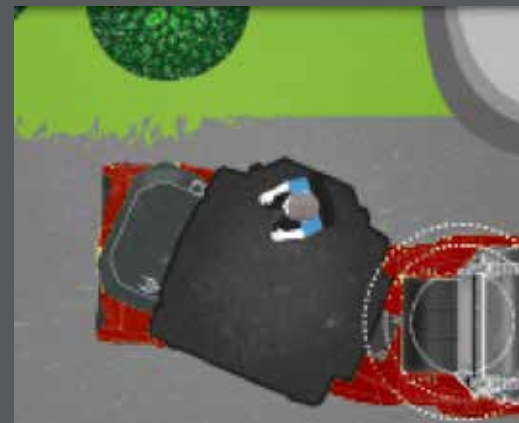
WEIGHT NEAR ROAD CENTER Along weak road edges you can keep the machines weight near road center.
