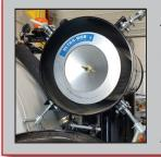
BAGHOUSE FILTRATION THE BAGHOUSE FILTRATION THAT FOLLOWS THE CYCLO-SEPARATOR FILTRATION HAS A WASHABLE AND REUSABLE FILTER THAT IS ACCESSED EASILY TO BE BLOWN OUT AND CLEANED AFTER USE.
